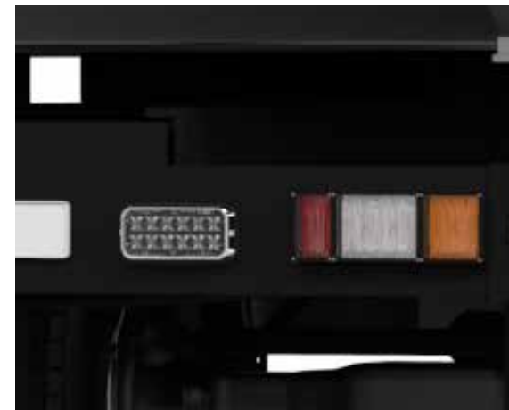
3. Wide Lux 7x3 can be synced to stop, tail & turn.
