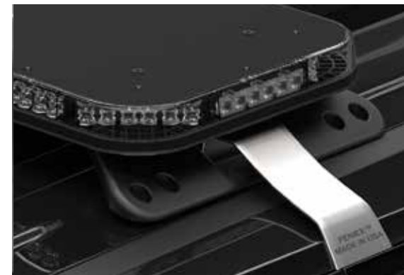
3. Fusion Light Bar with Hook Bracket Mount.
