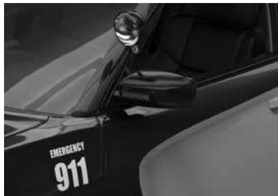
2. Vehicle specific Fusion Mirror Mount.
